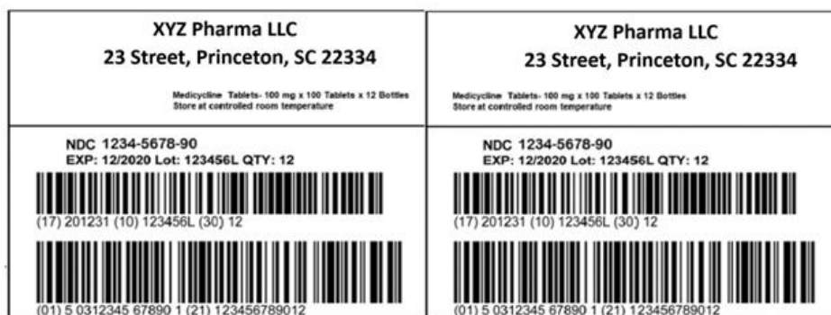
Fig. 2. GS1 1D Databar Liner Barcode required for Pharmaceutical Serialization
