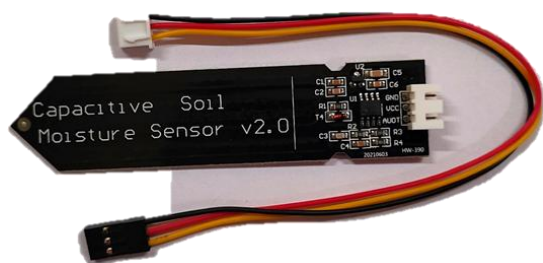
Fig. 3. Soil moisture sensors
