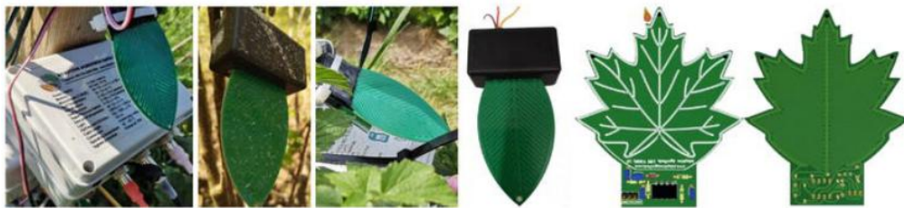
Fig. 7. ADP-AgroTech leaf wetness sensor (model ADP-LWS2020) with different leaf shapes based on capacitive method for determining leaf surface moisture and greenhouse condensation
