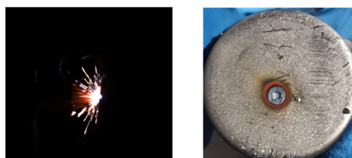
Figure 15. Arc traces under a circuit voltage of 200 V with different current direction: (a) charging; and (b) discharging.
