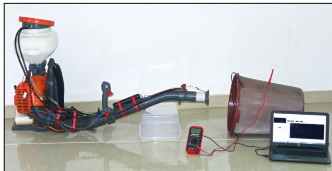
Fig. 8. Experimental set up for cloud charge measurement
