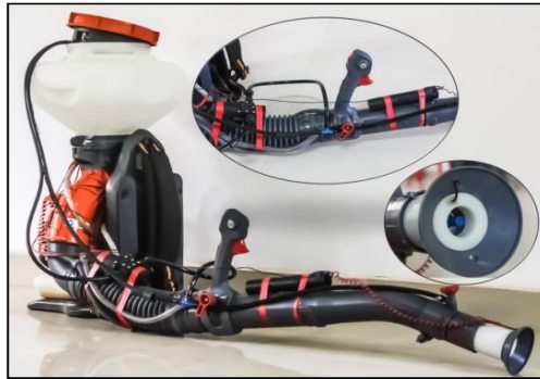
Fig. 7. Electrostatic charging unit with mist blower
