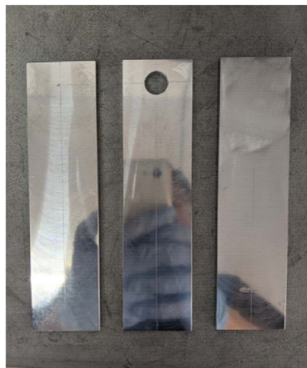
Figure 5. The left-most plate shows the substrate before drilling the hole. The substrate in the middle shows the location of the 12 mm diameter hole. The plate on the far right shows the hole after being filled up with cold-sprayed material and manually ground until flat on both sides.
