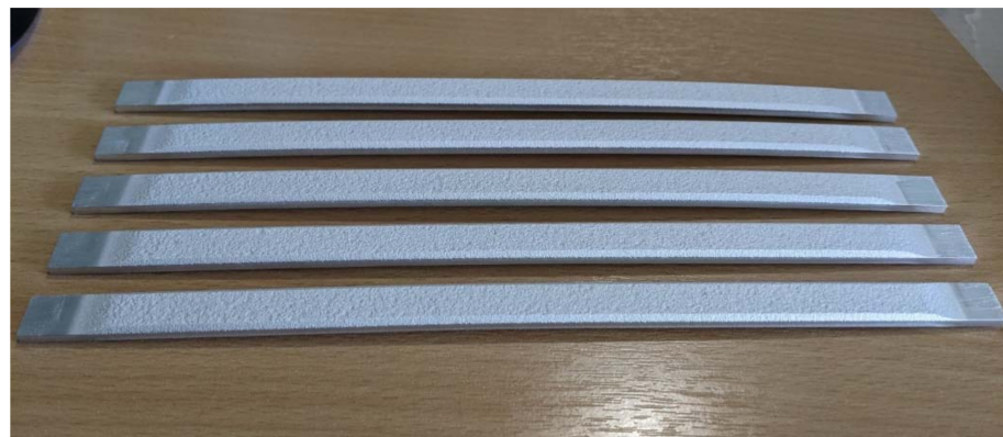
Figure 6. One set of aluminium 2024 bending test specimens (before bend testing).
