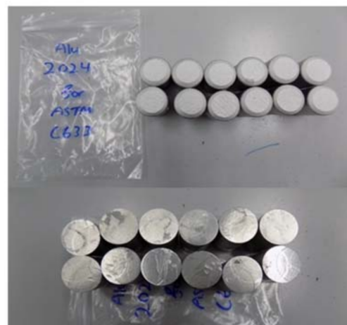
Figure 4. Al-2024 coating test specimens submitted for the adhesive bond strength test. The top image shows the coating top surface, while the bottom image shows the uncoated studs on the bottom side.
