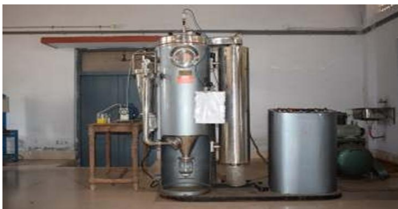
Fig. 1. Laboratory model pilot scale spray dryer
