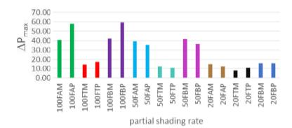
**Figure 4.** Power loss rate variation as a function of technology and shaded surface of the cell. Source: results of my work
