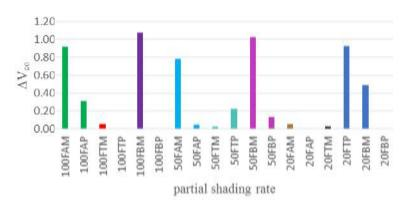
**Figure 5.** Rate of evolution of the open circuit voltage as a function of technology and shaded surface of the cell Source: results of my work
