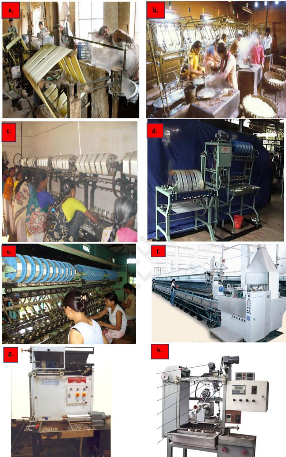
Fig. 1: a. Traditional charka b. Conventional domestic basin c. Conventional cottage basin d. CSTRI 6 end modified cottage basin e. Filature or multi-end reeling machine f. Automatic reeling machine g. Bobbin silk reeling machine h. CSTRI bulky raw silk reeling machine
