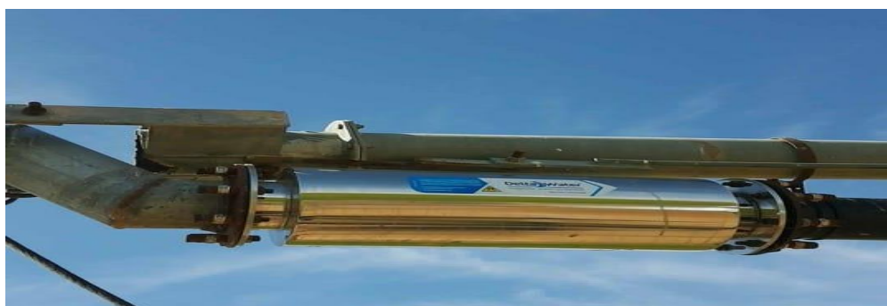
Fig 1. Magnetic system during irrigation water salinity study
