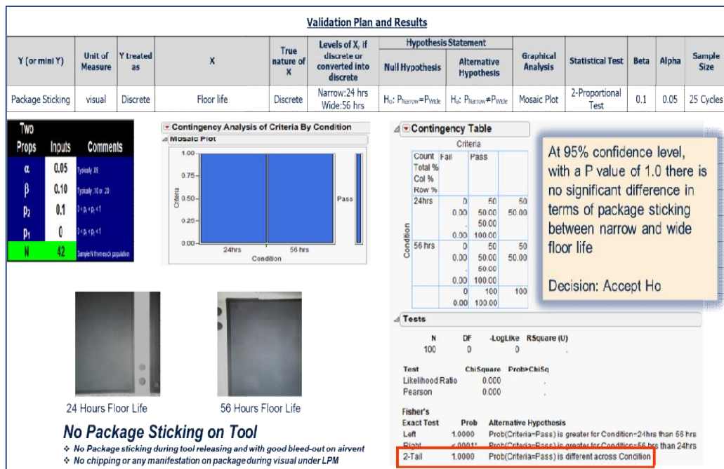
Fig. 19. Statistical validation result for package sticking
