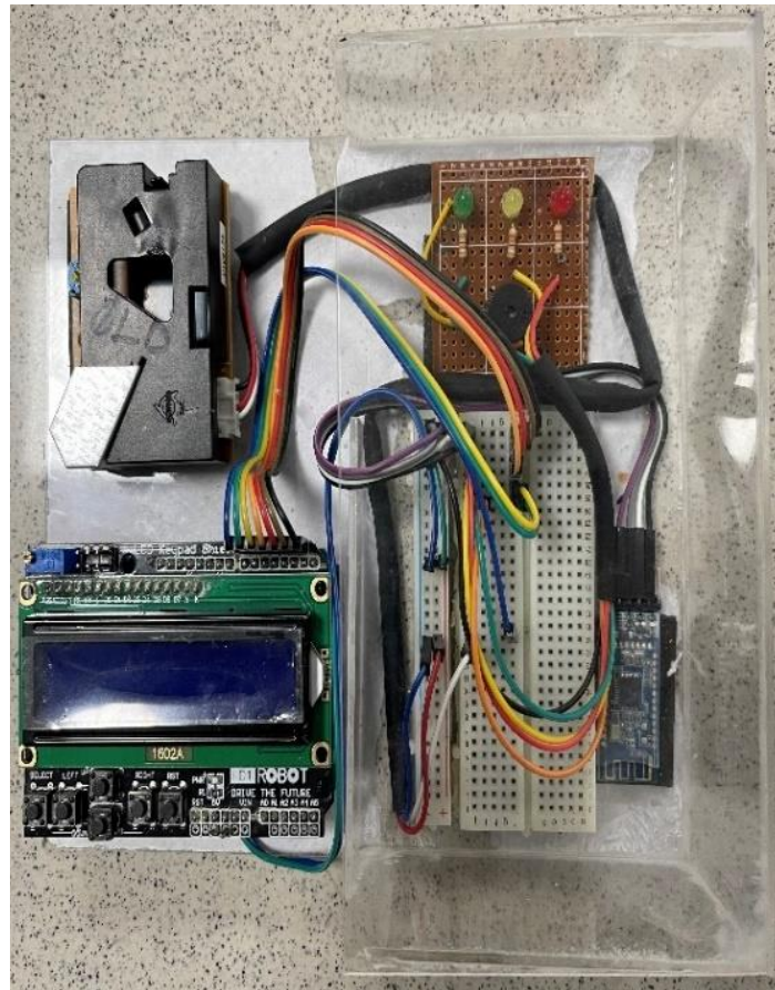
Fig. 6. Portable air quality detector using Arduino with acrylic cover.
