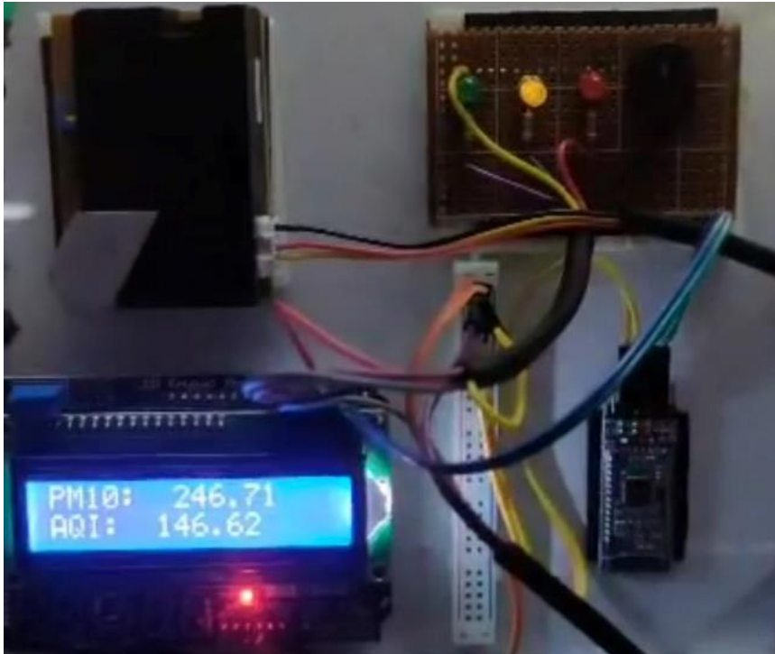
Fig. 7. Experimental AQI data is displayed in real-time on the LCD screen.
