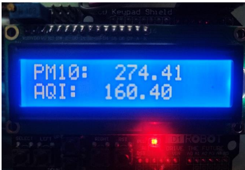
Fig. 8. Experimental AQI data is displayed in real-time on the LCD screen with a red LED indicator.
