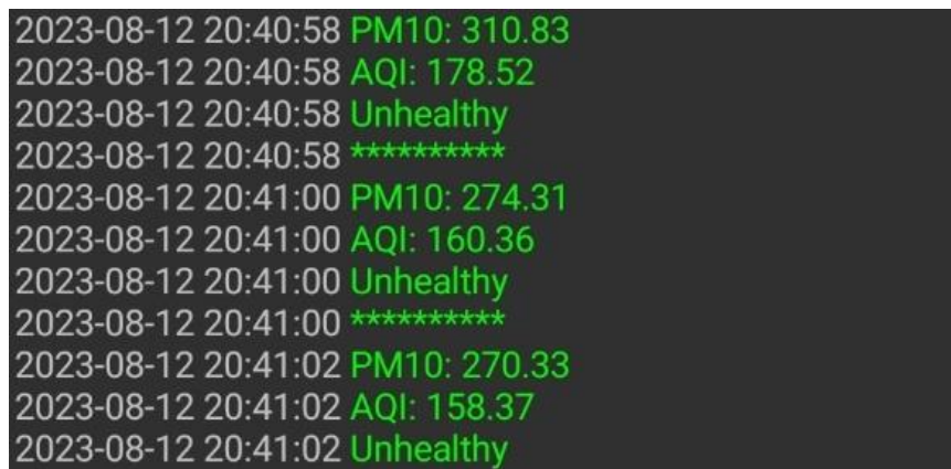
Fig. 10. Experimental AQI data is displayed in real-time on the Bluetooth-connected device including date and time.
