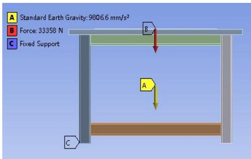
Fig. 4. Applied loads and boundary constraints diagram
