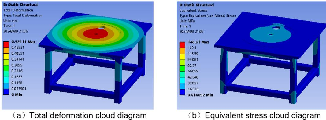
**Fig. 5. Total deformation cloud diagram and equivalent stress cloud diagram**
