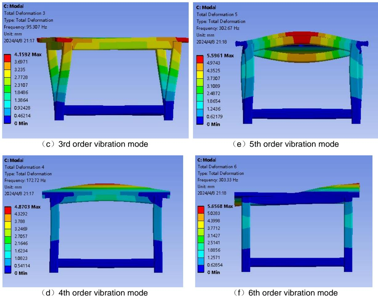
Fig. 6. 1st-6th order modal vibration pattern of the bracket
