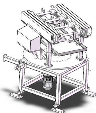
Fig. 1. Slewing unit model
