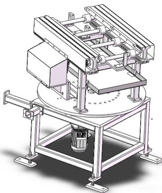
Fig. 1. Slewing unit model
