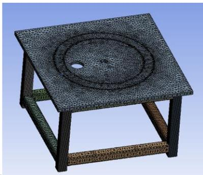
Fig. 3. Meshing of the model
