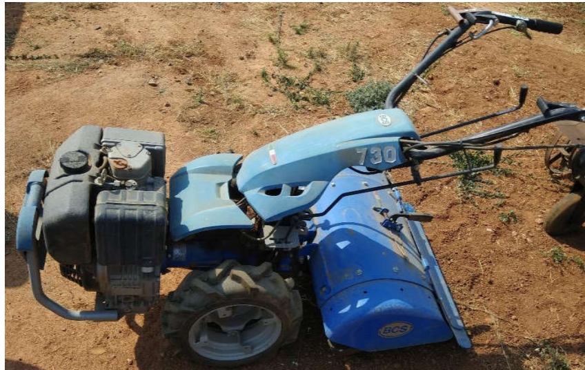
Fig. 1. Isometric view of power weeder
