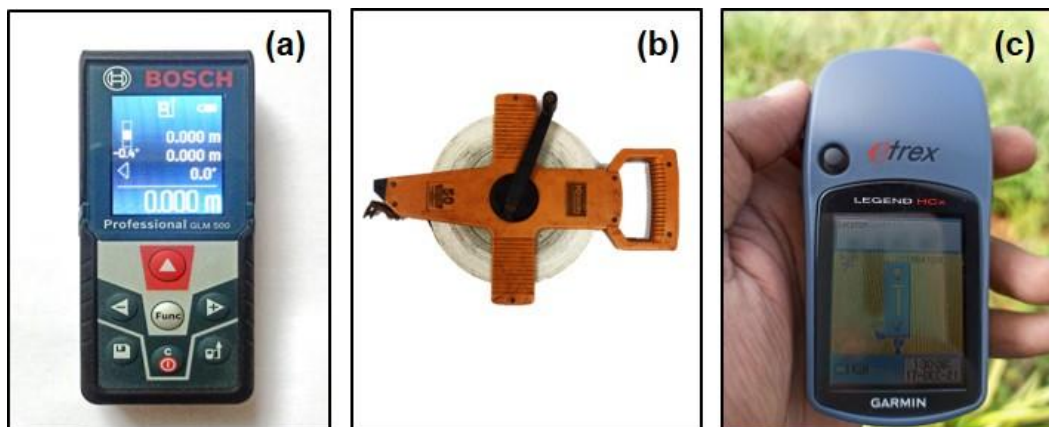
Fig. 2. (a) Laser rangefinder (Bosch Glim 500 Laser Distance Measurement Device), (b) Measuring tape (c) Geographical Positioning System (GPS)
