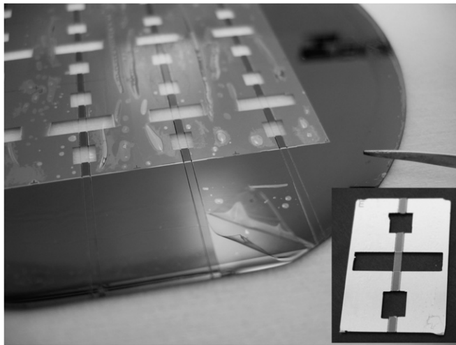
Figure 5. Picture of PU tensile test specimen fabrication: peeling off the polyurethane layer after the KOH etching process step (in insert: finished specimen).
